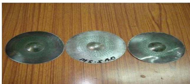
**Fig. 2** MS samples after formability test
